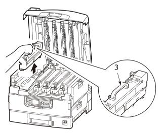
NOTE Avoid the fuser unit bumping to the LED head.
