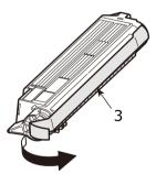
**7.** Holding the toner cartridge with the tape face down, match the hole (4) of the toner cartridge on the protrusion (5) of the image drum and carefully lower it on the image drum.
