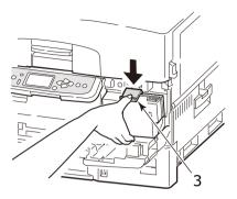
**4.** Remove the waste toner box (4) from the printer.
