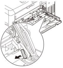
**5.** On the left side of the multi-purpose tray, move the lever (5) located on the connecting part between the printer and multi-purpose tray to the position shown.
