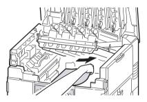
**4.** If paper is jammed in the fuser unit, push the lock lever (3) in the direction shown to release the unit.
