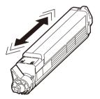
**6.** Place the toner cartridge on a flat surface, and peel off the adhesive tape (3).
