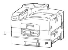
2. When the display panel shows that you can either turn off or restart the printer, use the On/Off switch to turn off the printer.
