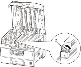
**3.** Lift the toner cartridge carefully and remove it from the printer.
