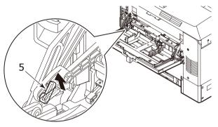
**6.** Lift the multi-purpose tray slightly with the left hand, and push the lever inward and release it with the right hand.
