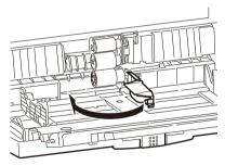
**11.** Holding the connecting parts between the printer and multipurpose tray with both hands, lower the cover.
