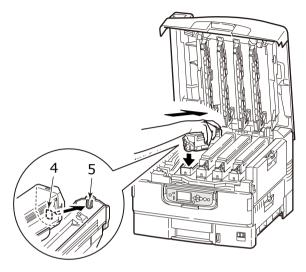
**8.** Pressing gently down on the toner cartridge to ensure that it is firmly seated, lock it by turning the blue lock lever (6) to the direction of the arrow until it stops.
