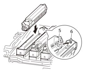
**11.** Pressing gently down the toner cartridge to ensure that it is firmly seated, lock it by turning the blue lock lever (7) to the direction of the arrow until it stops.
