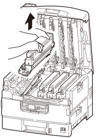
**3.** Turn the blue lock lever (2) of the toner cartridge to the direction of the arrow until it stops to release the lock.
