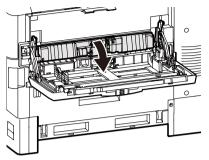
**12.** Lift the right side of the multi-purpose tray slightly, and fit the protrusion of the lever (6) as shown.
