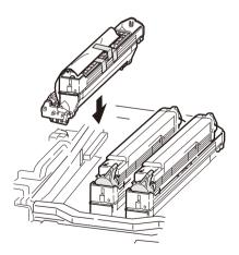
**5.** Pinch the both ends of the protective sheet with the thumb and index finger while holding down the image drum cartridge with other fingers, and pull out the protective sheet to the direction of the arrow.
