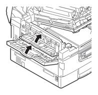
**10.** Return the image drum basket (9) into position and check it is locked.
