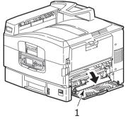
**3.** Remove Tray 1 completely from the printer.
