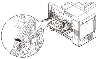
**16.** Slide the paper guides to their outermost positions, and fold the paper support section.
