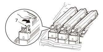
**12.** Open the LED head guards (8) and gently wipe each of the four heads (9) with an LED lens cleaner or soft cloth. Move the cleaner as shown, using a clean section of the cleaner with each pass. Be careful not to damage the guards.
