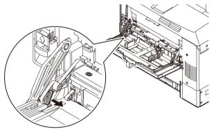
7. Move the released part to the printer side. The cover lifts and the paper feed rollers appear.
