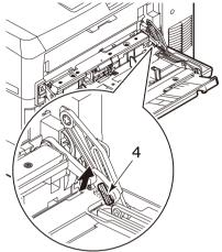
**4.** Lift the multi-purpose tray slightly with the right hand, and push the lever inward and release it with the left hand.
