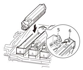
**10.** Pressing gently down the toner cartridge to ensure that it is firmly seated, lock it by turning the blue lock lever (7) to the direction of the arrow until it stops.
