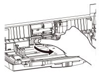
**9.** Wipe the 3 paper feed rollers with a soft cloth lightly moistened with water.
